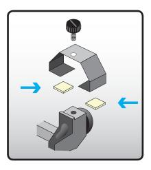
The **Carriage** contains **2 brackets** on the front edge that hold **4 felt pads** onto Velcro inserts.
