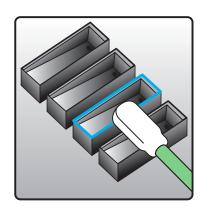
**Moisten** a swab as done for the wiper blade cleaning, and swab the edges of the cap rubber.
