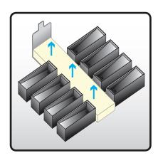
When needed, you can replace the **cap felt** sitting in between the two sets of four caps.
