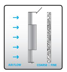
The fan filter collects the mist from the print head spray from the exhaust provided by the fan.
