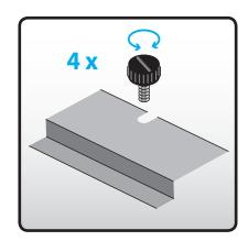
**Loosen** the four black thumb **screws** (do not remove) on the encoder cover, and remove the cover.
