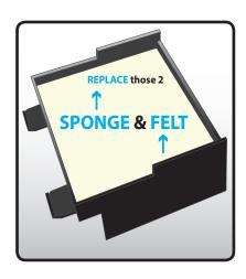
Insert the **felt** into the **flushing plate**.
