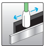
The wiper **cleans** the underside of the **print heads** to allow the **nozzles** to fire properly. The wiper is cleaned by passing across the **wiper cleaner**.
